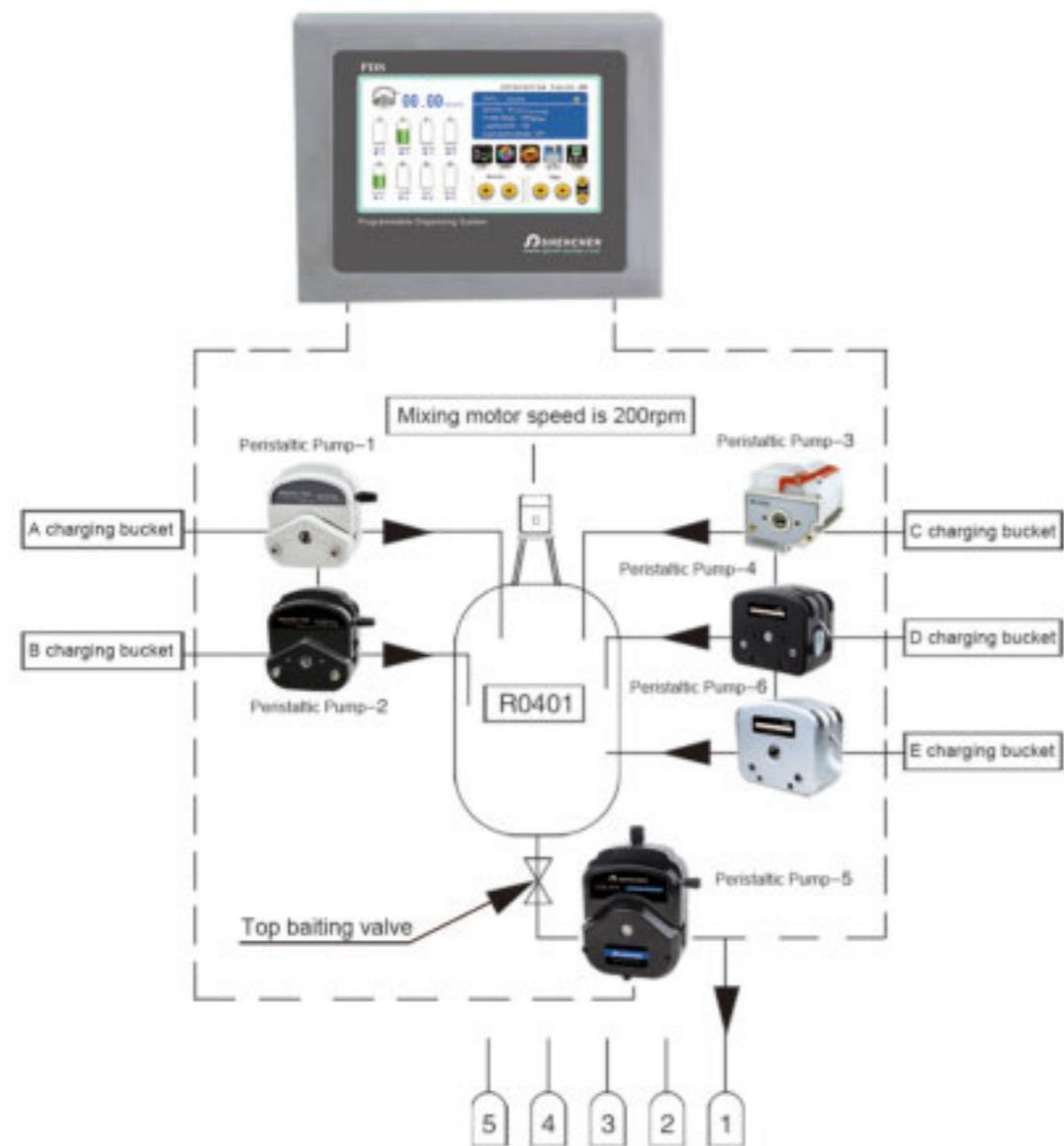
**Application 1 Chemical industry:** Reactor liquid adding, dispensing and washing, with different volume and adding liquid according to preset order.
