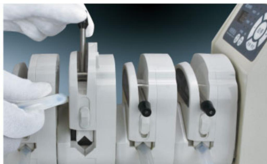
YZ Series pump head has wide application, and is usually used together with many kinds of analytical instruments. According to the different technical requests, it can adopt different motors to drive, such as stepper motor, DC motor, synchronous motor, AC gear motor, etc. Stack up several pump heads can increase the flow rates.
