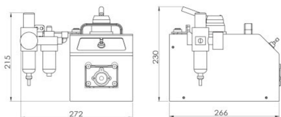
Non-working status dimension drawing (Unit: mm)
