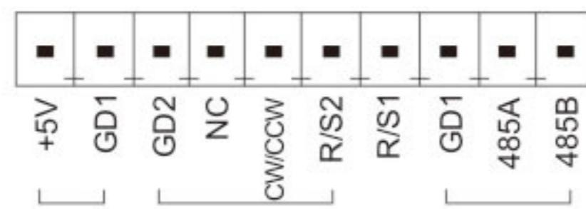
DF600plus External Control Schematic Diagram
