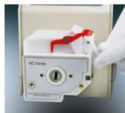
B. After that, the cartridge can be taken out lightly.
