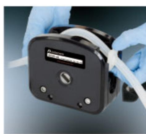
3. Install the upper block, put down the levers to lock the block.
