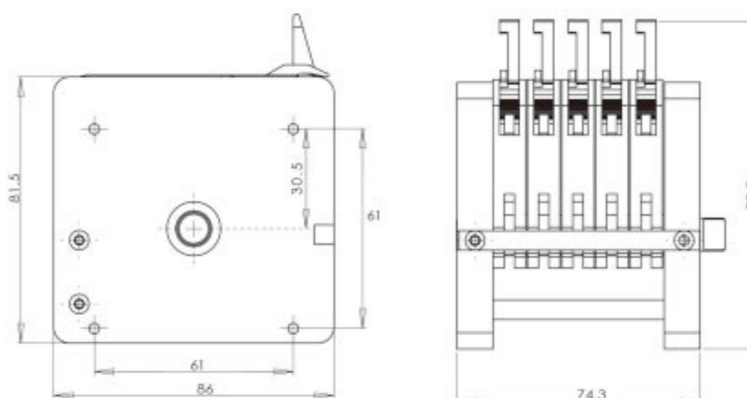
**Note:** Increasing or reducing one channel, the pump head size need to increase or reduce the thickness of one cartridge.
