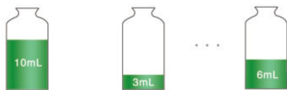
In independent working mode, each unit working independently, can fill different volume.
