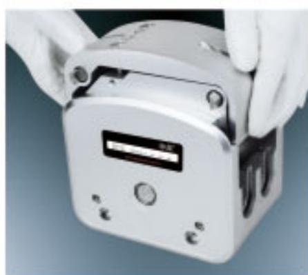
2.Put the tubing with tubing clamp into pump housing.
