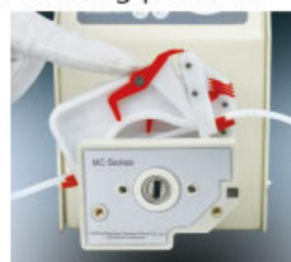
E. Turn the spanner counter-clockwise to make it reach the lever.
