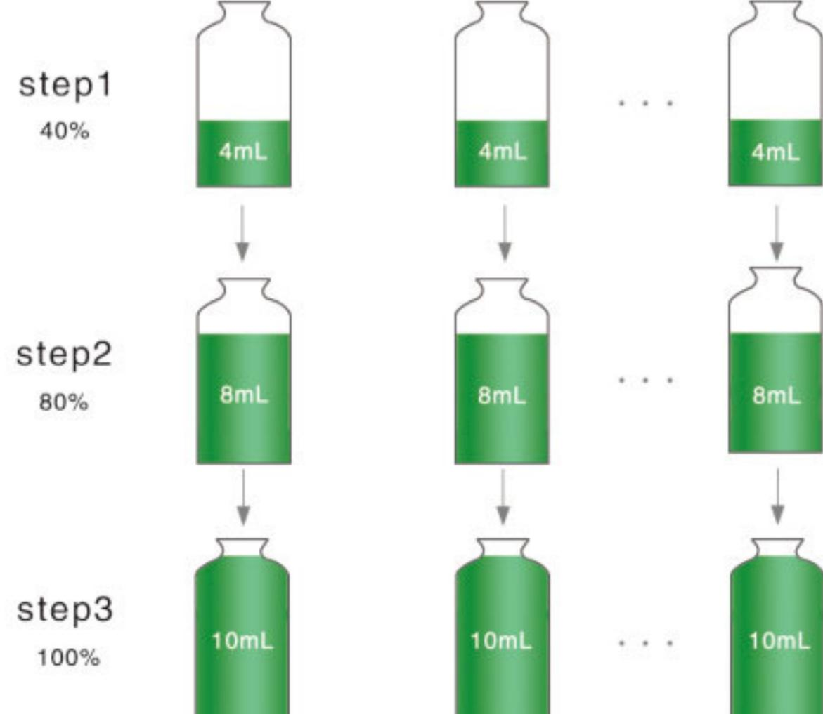
In independent working mode, each unit can finish filling process with multiple different filling volume. This function suitable for prevent fluid splashing and foaming. This process can also repeat many times, achieving complicated dispensing function.
