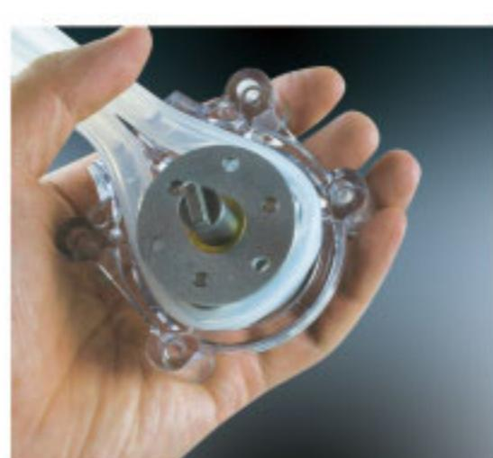
C. Tighten the tubing aptly, and load the other half pump head body.
