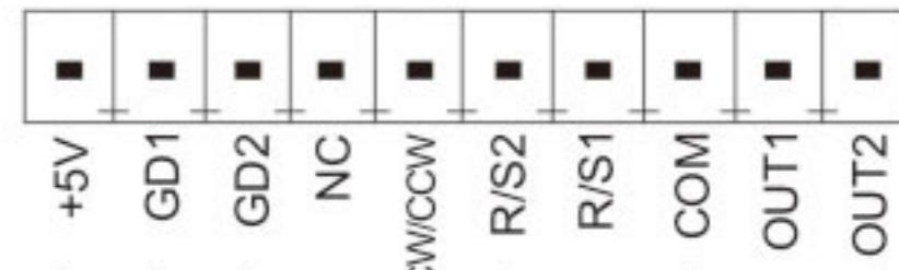
DF600 External Control Schematic Diagram
