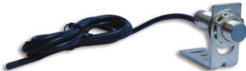
When applied in the dispensing line, it can detect whether there is filling bottle in the production line. When the bottle approach the sensor side, the switch action will be made without any mechanical contact or pressure, thereby providing filling control order to the pump. In the same way, when no filling bottle is detected, the stop filling control order is provided to the pump.
