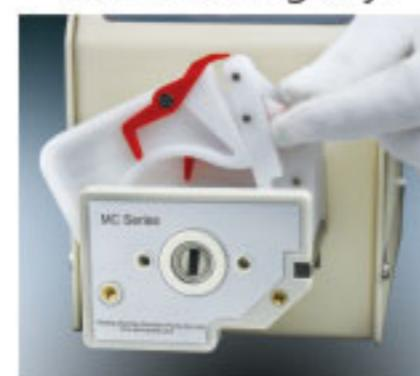
C. Install the tubing and confirm the working position between two adjacent clamps.
