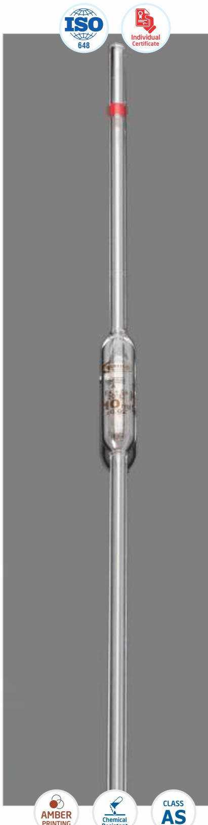
Glassco volumetric pipettes are manufactured in compliance with DIN ISO 648 standards. These pipettes are calibrated to deliver (TD, EX) + 20°C.
